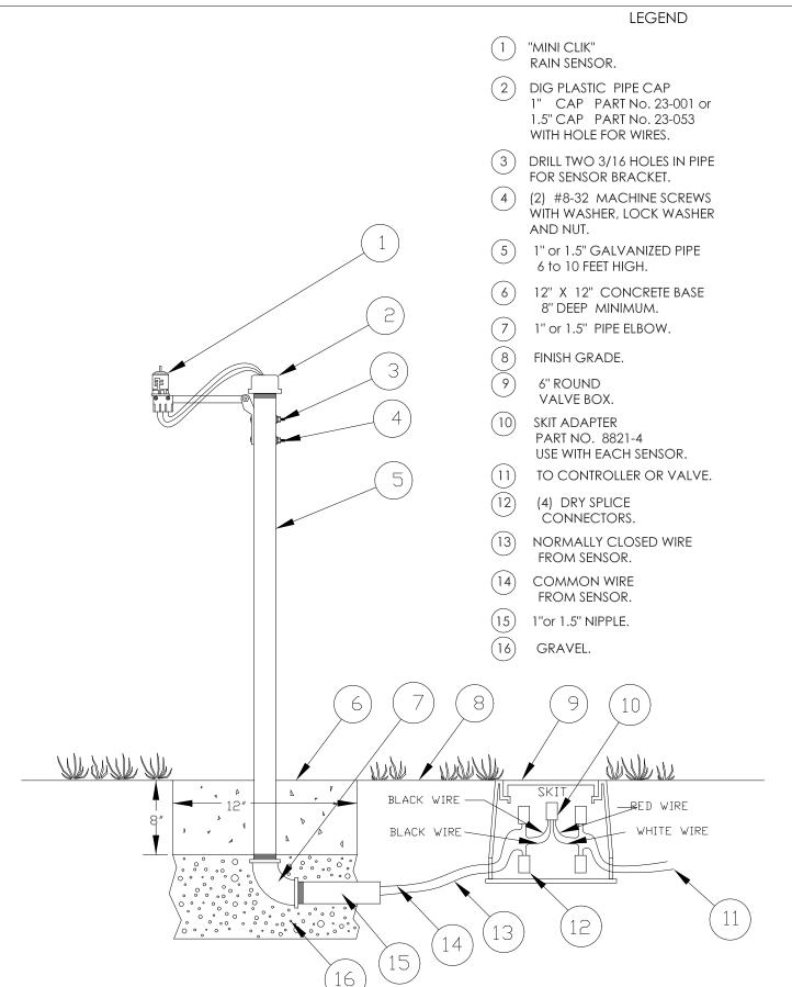
RAIN SENSOR ASSEMBLY (COLUMN MOUNTED)
