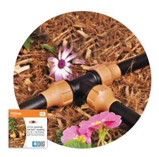
DIG's universal nut lock<sup>™</sup> drip fittings are used to connect any 1/2" to 5/8" poly tubing and dripline with .620 OD to .710 OD. Used by both DIY homeowners and professionals, the fittings are made of high-impact plastic for long life without the need for glue.
