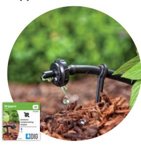
Pressure compensating or flow regulating drippers continuously adjust to varying water pressures, ensuring a constant flow rate from each drip emitter, regardless of water pressure fluctuations or varying elevations along the line. They are the most accurate and trouble-free drippers.
