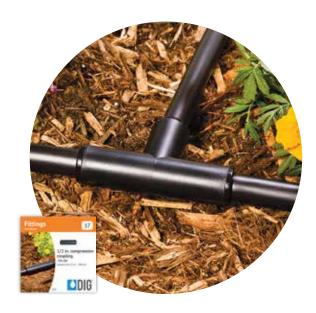
Constructed of molded UV-resistant, high-impact plastic, DIG's compression fittings provide a secure water-tight fit without the need for glue or cement. Utilizing spin-weld technology, the ABS bodies are assembled with a polycarbonate insert that's welded into place. With the many sizes of 1/2" poly tubing, DIG provides compression reducing couplings so that whatever size of tubing is used can be integrated into the system.
