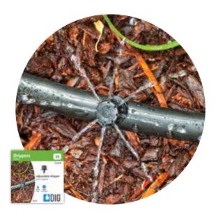
Easily adjust the top flow dial of these drippers from 0-14 GPH and the radius of their wetting pattern to accommodate plants as they grow, without needing to change or add more drippers. The adjustable dial can also be removed to flush and clean the dripper.
