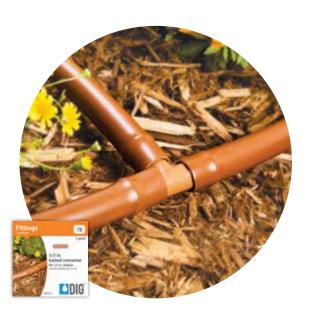
The brown 1/2" barbed drip fittings are used in the installation of DIG's 1/2" pressure compensating dripline or poly tubing. They are inserted into the tubing, unlike the compression fittings which are installed over the tubing. Using a double barb and UV-resistant, highimpact plastic, these barbed fittings provide a reliable water-tight fit without using glue.
