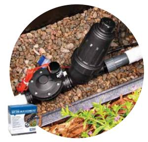
The automatic valve assembly kit automates a drip irrigation zone, provides protection to the drip emitters and micro sprinklers from particles that may enter the system, and reduces or regulates the incoming pressure to the appropriate operating pressure of 25 PSI, which is the recommended operating pressure for a drip irrigation system. It easily connects to any existing alternating-current (AC) timer.
