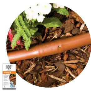
Sophisticated cylindrical 1 GPH drippers are preinserted in the tubing every 18". Dripline provides one of the easiest drip irrigation installs; simply layout the tubing and connect to your water source. Each dripper is pressure compensating to provide a consistent flow throughout the length of the line.
