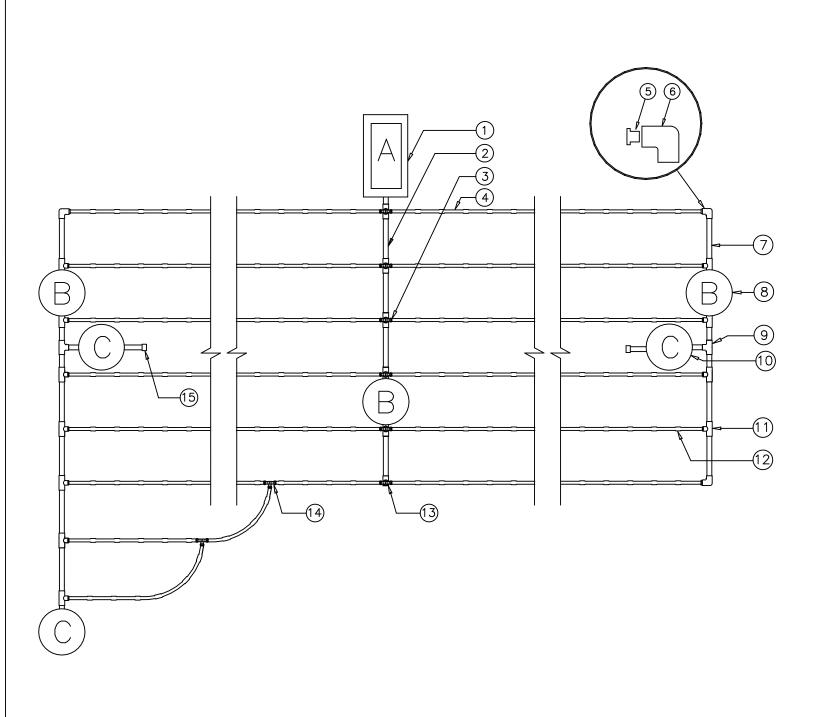
17 MM WITH CV PC DRIP LINE FOR SUBSURFACE INSTALLATION
