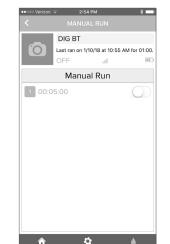
The Manual Run screen allows for manual operation of the timer. It can be reached by selecting the Manual Run button on the bottom right of the screen. Modify the duration by tapping on it and start and end the run by tapping the button to the right.
