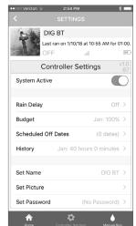
The timer's Settings screen contains everything else needed to fully control your irrigation system. It can be reached by selecting the Controller Settings button 🚺 on the bottom of the screen.
