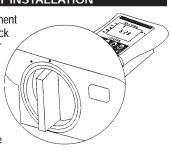
IMPORTANT: To replace the battery compartment cover, insert it with the handle in the "11" o'clock position to avoid possible cover guide pin breakage.
