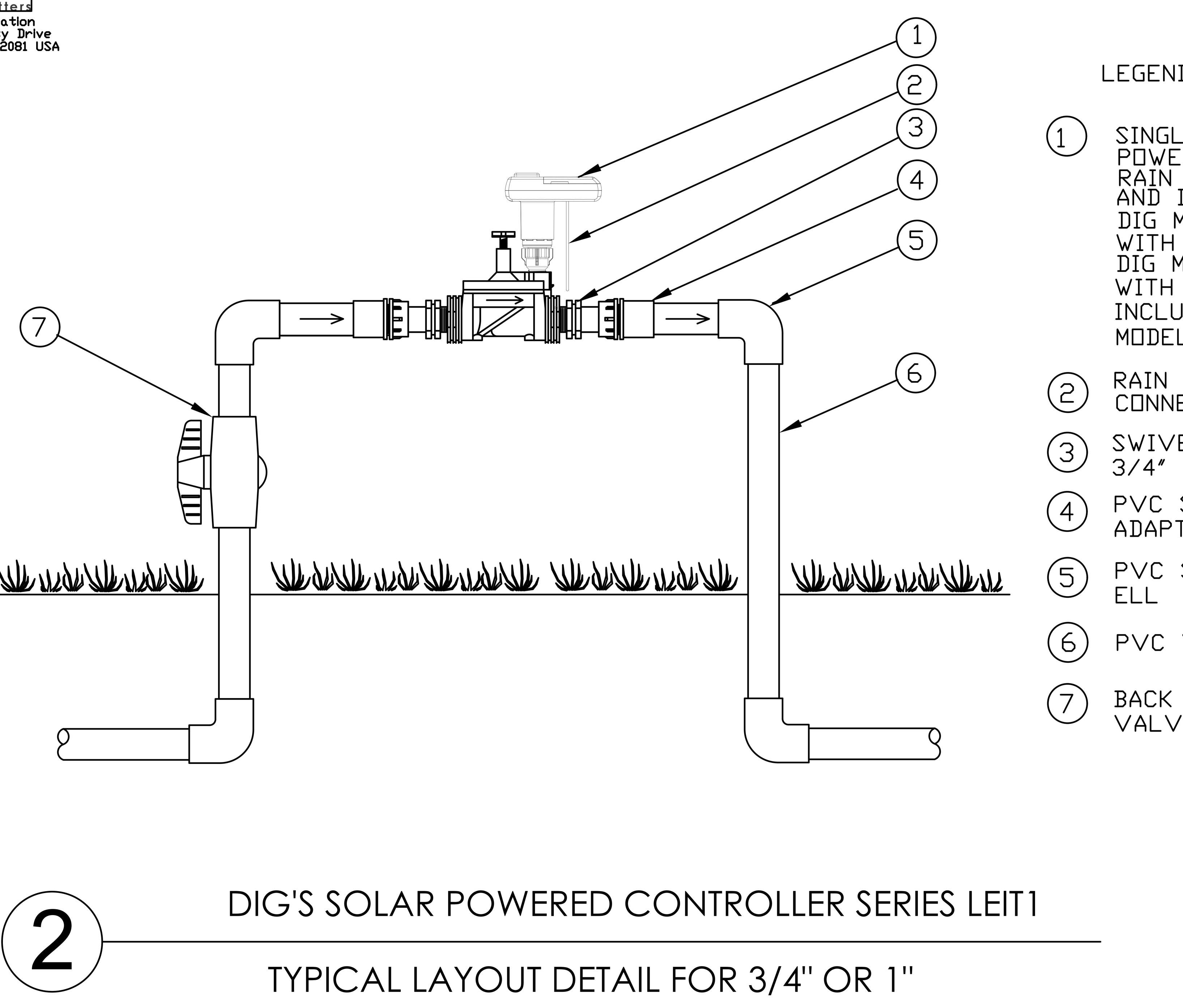
SINGLE STATION SOLAR WITH POWERED CONTROLL RAIN SENSOR CONNECTION AND INLINE VALVE (IP68) ILV-075DIG MODEL# INLINE VALVE DIG MODEL# ILV-100-E111INLINE VALVE INCLUDING VALVE ADAPTER MDDEL: 30-920 RAIN SENSOR WIRE CONNECTION SWIVEL FITTING DIG MODEL 3/4" 23-004, 1" 23-003 PVC SCH 40 MALE PVC SCH 40 90 DEGREE PVC VERTICAL LINE BACK UP NPT PVC BALL
