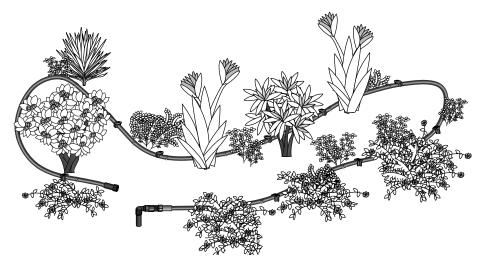
Open the system valve and make sure that the PC dripline provides the coverage desired, and if necessary, move the PC dripline closer to the plants.
