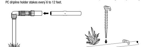
compression side while moving it from side to side and secure the PC dripline to the ground by installing the
