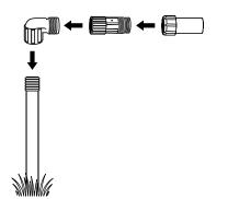
4. Turn the water on and flush the line thoroughly. Turn the water off and close the end of the line with the hose end connector forcing the end of the PC dripline into the adapter compression side while moving it from side to side
