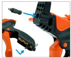
Secure the tip by pulling up the lock.
