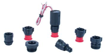
DIG's S-305DC is an encapsulated, watertight, two-way magnetic latching solenoid that requires minimal power to operate. The S-305DC is used with the 710AP-XXX battery operated controllers and others. With seven solenoid adapters available, the S-305DC can replace conventional solenoids on most valves, enabling DIG controllers to operate most brand name valves using DC power.
