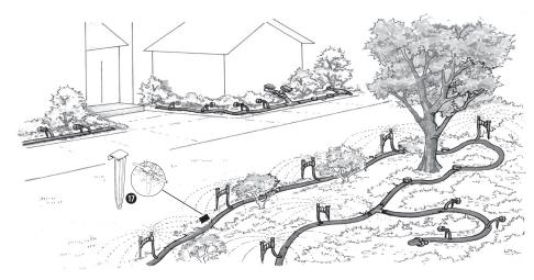
To install your 1/2" fittings, cut the poly tubing with a hand pruner or scissors, being careful to keep dirt from entering the line. Push the poly tubing into the fitting by wiggling it as you apply force
