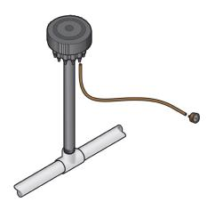
4. Secure the micro tubing near the plants by attaching the V-stake towards the end of the micro tubing, taking care to space the drippers appropriately.
