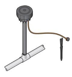
5. Use the rubber caps provided to close all unused outlets. Do this by unscrewing the cover and removing the Mini-Disk filter. Then, press the rubber caps into the unused outlets, and re-install the Mini-Disk filter and cover. Tighten the cover by hand.
