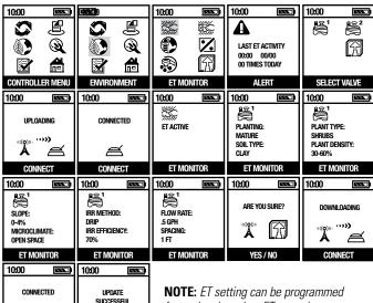
**NOTE:** ET setting can be programmed for each valve when ET setup is changed to Active and can be overridden at any time.
