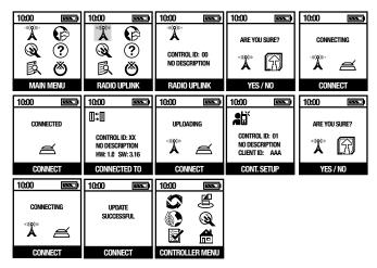
**Step 1:** Make sure the LEIT-2ET controller is out in bright light to harness light energy used to power the controller. It will take approximately thirty (30) minutes, or less, in direct sunlight. Do not connect sensor wires at this time. Wait until controller is charged and ready to be assigned an ID.
